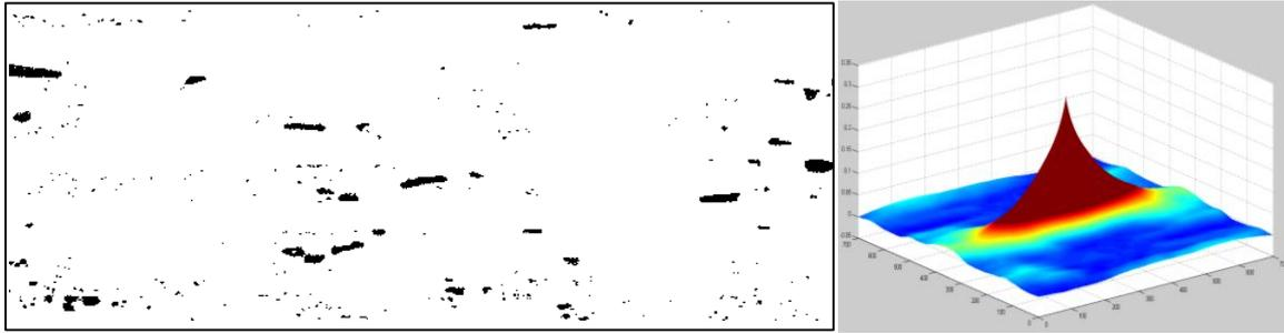
**Figure 1:** Thresholded micrograph of voids (left), 2-point correlation showing density and directionality of void clusters.
