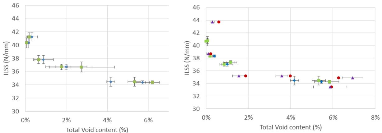
**Figure 2:** Local measured void content vs. ILSS, averaged across rows (left) and further split into columns (right).
